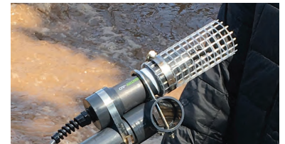
Figure 2.3 Protected drop-in mount
